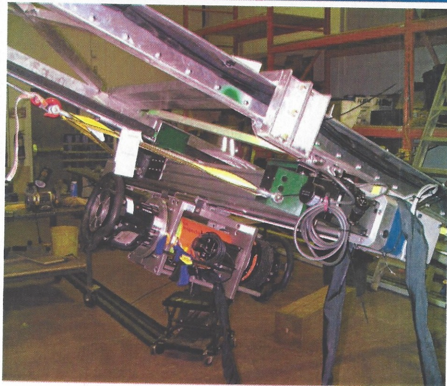
Three degrees of motion: the orange X-ray tube rotates, and also slides side to side and up and down. Photo: Acuren
